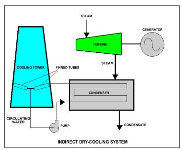
Figure 4–7. Indirect Dry Cooling
