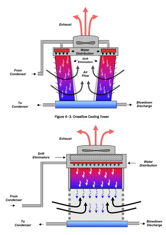
Figure 1-4. Counterflow Cooling Tower
