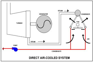
Figure 4-6. Air Cooled Condenser ("Direct Dry")
